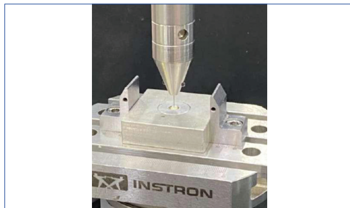
[Table/Fig-14]: Push Out Bond Strength (POBS) test using universal testing machine (Instron).
